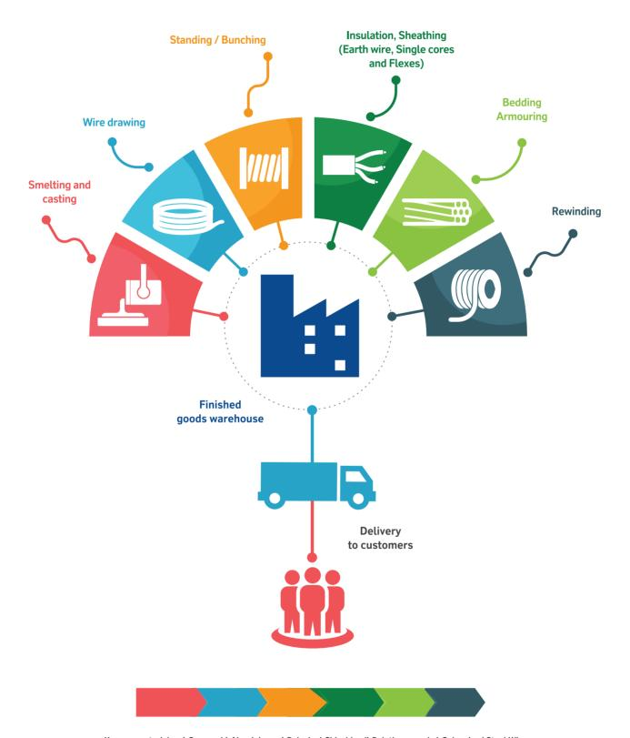
Key raw materials: a) Copper, b) Aluminium, c) Polyvinyl Chloride, d) Polythene, and e) Galvanized Steel Wire
